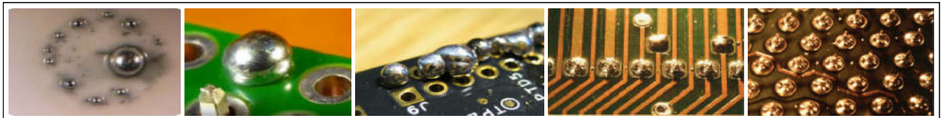
Various examples of solder ball formation during soldering with normal type Feeding Unit
