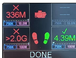
Wrist Strap and left foot wearing is over limit Right foot wearing is OK
