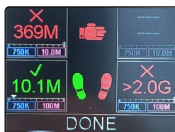
Wrist Strap and right foot wearing is over limit Left foot wearing is OK
