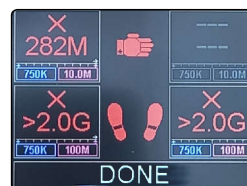
All ESD wearing wrist strap as well as foot wearing are over limit
