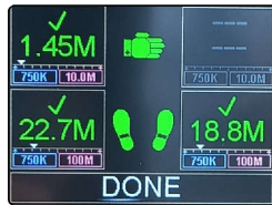
All ESD wearings wrist strap as well as foot wearing are OK
