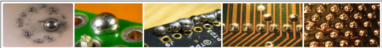
Various examples of solder ball formation during soldering with normal type Feeding Unit
