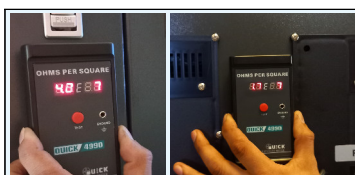
Complete Cabinet is ESD Safe including Housing (painted with ESD Grey paint) and Castor Wheels
