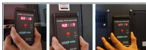
Complete Cabinet is ESD Safe including Glass windows, Housing (painted with ESD Grey paint) and Castor Wheels
