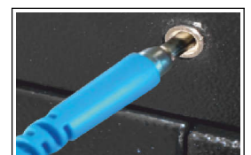
Wrist Strap Terminals for additional ESD Safety
