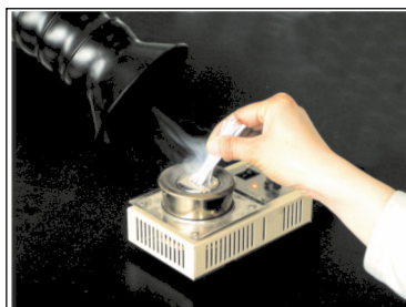
Solder fumes extraction during hand soldering on PCB & Solder Pot tinning
