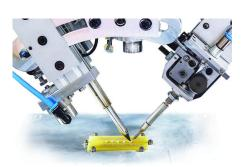
Soldering Robot that has two independent mechanisms one feeds the soldering wire to the joint (to be soldered) directly and the other mechanism performs solder on to the PCB yielding more efficiency, reliability and accuracy.
