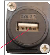
in-built USB Port for Data Logging (with customer's computer)
