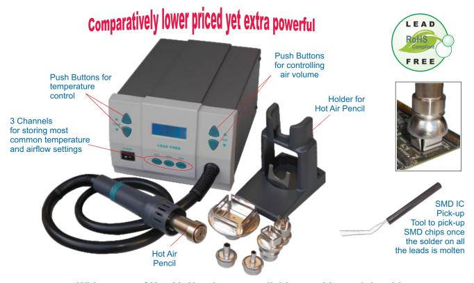
Wide range of Hot Air Nozzles are available to solder and desolder Fine-Pitch QFPs, PLCCs and SMD ICs up to 42.5x42.5mm size
