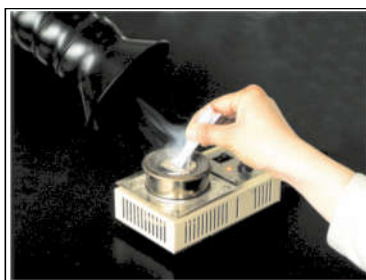
Solder fumes extraction during hand soldering on PCB & Solder Pot tinning
