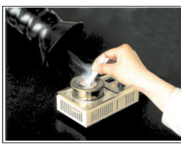
Solder fumes extraction during hand soldering on PCB & Solder Pot tinning
