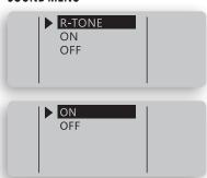
Sound menu is used to change the sound setting for measurement confirmation.
