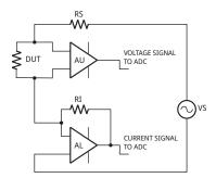
Voltage across the component is generated by the test signal source Vs. Both the amplitude and frequency of Vs can be set. The voltage is applied to the device under test (DUT) through the source resistance Rs. Current flows to the virtual ground of the current amplifier AI, and through the current conversion resistor Ri. The output of AI provides a signal proportional to the current, I\*Ri.
