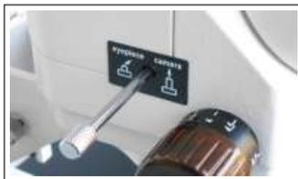
**Switch between Video and Eyepiece View**
