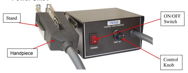
Power Unit: Power Unit has a low-voltage, high ampere, variable output. There is control knob for adjusting Output voltage which leads to adjusting Heating of Handpiece.
