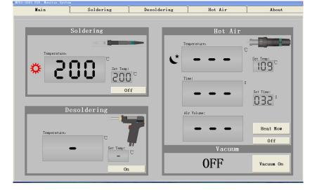
1.3 The computer and the machine online steps:1.3.1 Install a good driver, will be USB line into the computer;1.3.2 Open the device manager, and then open port;
