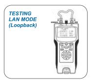
Testing from Main RJ45 Connector to Loopback RJ45 Connector
