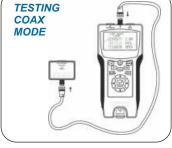
Testing from F Connector to Remote F Terminator Connector
