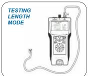
Testing from Main RJ45 Connector to open cable on other end
