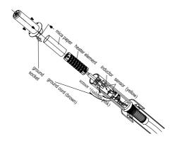
$\triangle$ Note: Avoid invalidate the ground cord when replacing the heater element.
