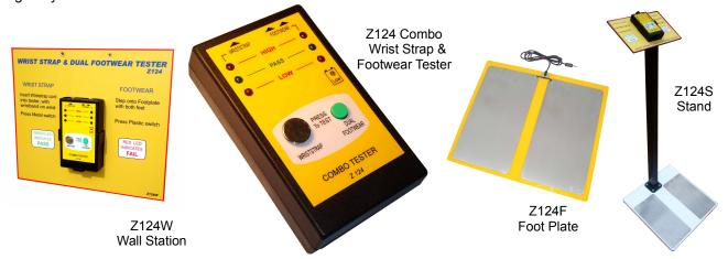
In order to protect sensitive electronic components, the maximum wrist strap resistance should not be more than 10 meg ohms and footwear resistance should not be more than 35 Mega ohms. On the other hand, the resistance should not be less than 0.75 Mohm as protection to the wearer from dangerous levels of voltage and current flow.
