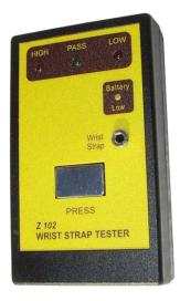
In order to protect sensitive electronic components the maximum strap resistance should not be more than 10 meg ohms. On the other hand, the path to ground should have atleast 750 kiloohm resistance, as protection to the wearer from dangerous voltages and levels of current flow.
