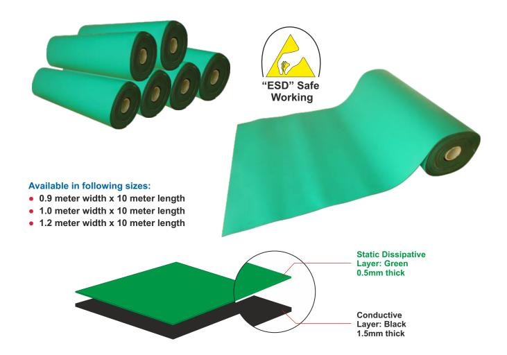
2-Layer ESD Rubber Mats have a top layer of static dissipative rubber layer laminated to a black conductive rubber bottom layer. Surface resistivity of the top layer is 10° ~ 10° ohm and the bottom layer is 10° ~ 10° ohm. The 2-Layer ESD Rubber Mat material offers excellent resistance to oil, grease and most common solvent. These Mats provide ESD safe working for Workstations, used in electronics assembly/repair/field's service.
