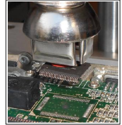
in-built Vacuum Pick-up lifts large SMD IC gently without damage to SMD pads PCB
