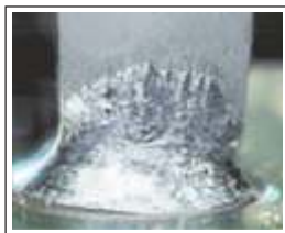
SMD Pas Solder Lift-off Inspection
