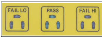
Nine Test Lights for Wrist Strap and Foot Wear testing (3 Pass Green, 3 Fail Low & 3 Fail High)
