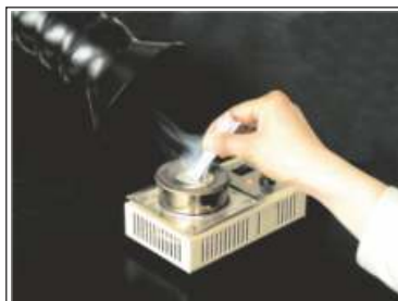
Fumes Air Purification during hand soldering on PCB & Solder Pot tinning
