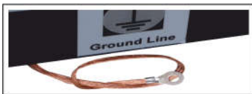
Grounding Line is provided at back side
