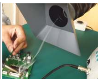
Fumes Air Purification during hand soldering on PCB & Solder Pot tinning
