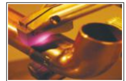
Carbon block electrodes can be easily shaped, allowing the user to customize the Hand Piece as per their specific application requirements.
