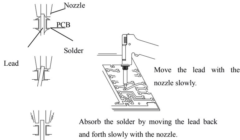
4. **Problems during de-soldering:** If solder remains, it must be soldered again and the de-soldering process repeated as above.
