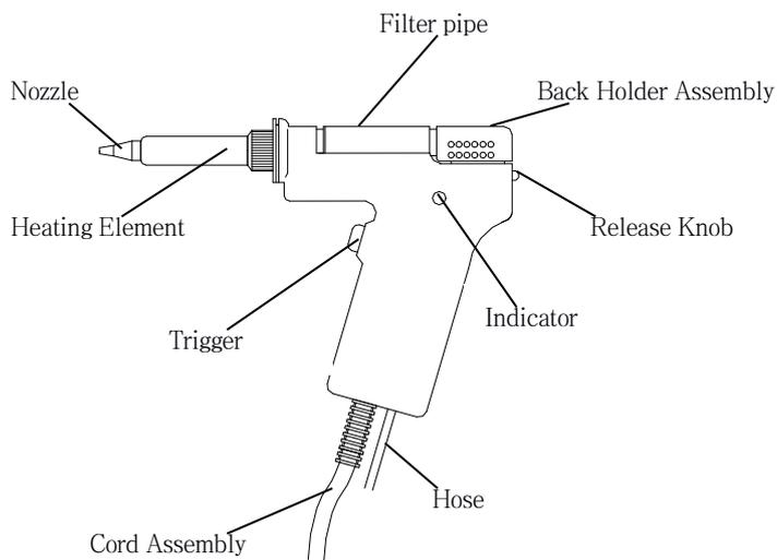
**Nozzle:** Transmits heat for melting solder. It is entrance of the melted solder. Expendable part.
