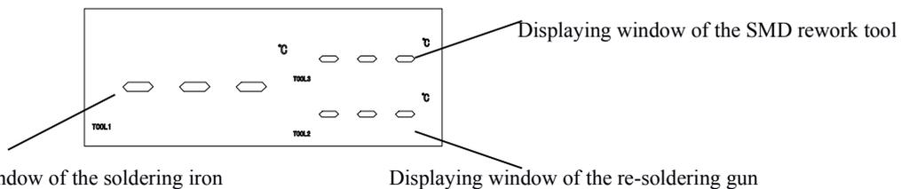
2. In the whole displaying window, click “TOOL1” or “TOOL2” or “TOOL3” key into the single displaying. In the single displaying state, the unit will return the whole displaying window if without operation about 5seconds.
