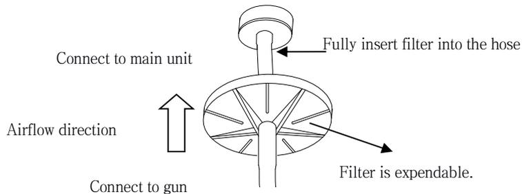
**Note:** The external filter has connection orientation, and it must be connected according to the mark, otherwise affect suction.
