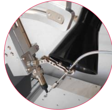
Fume Absorber fitted very close to Soldering Head to extract the fumes generated while soldering
