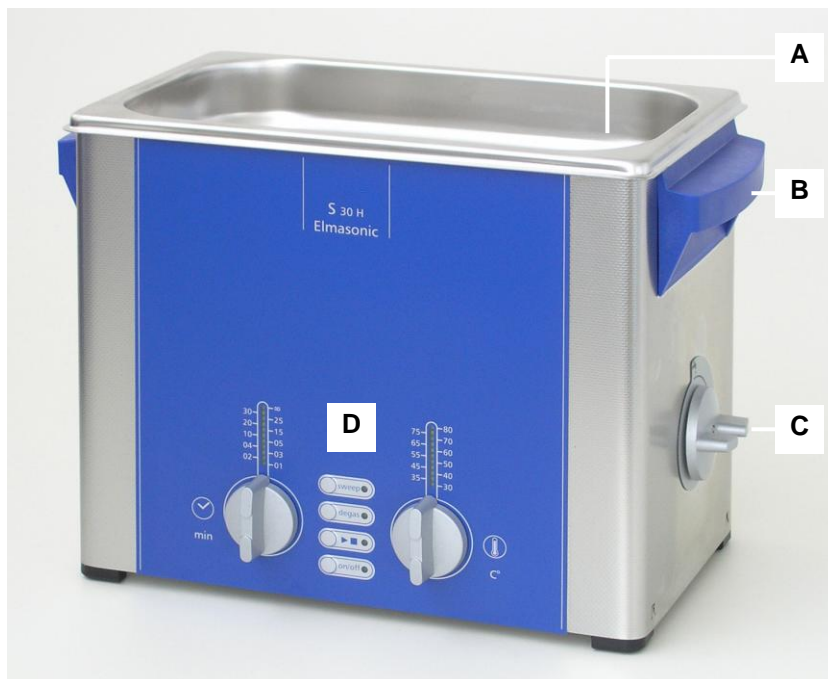
Illustration 4.4 Front view / side view Elmasonic S 30 H
