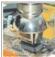
Large SMD Desoldering
