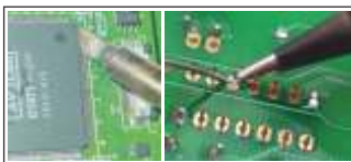
Soldering Station Model DSS36 for soldering SMD ICs and PTH components
