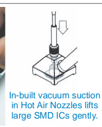
HAP 200 Hot Air Pencil with WRK Nozzle
