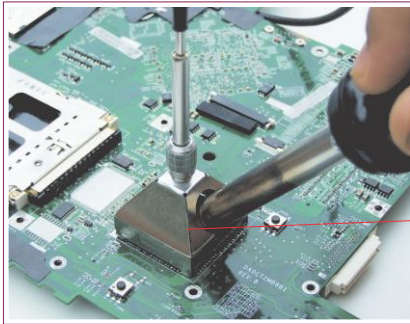
HAP 200 Hot Air Pencil provides Static Free hot air
