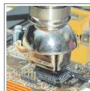
Large SMD Desoldering
