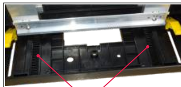
Smooth sliding easy PCB size adjustment
