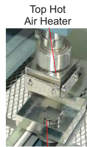
Top Hot Air Heater Bottom Hot Air Heater
